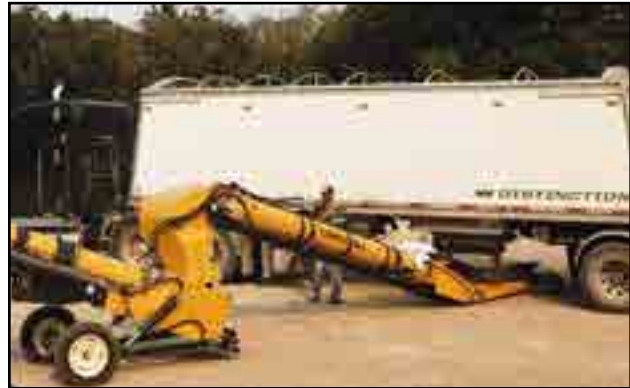
Fig 55 - Trailer unloading into swing-out conveyor
