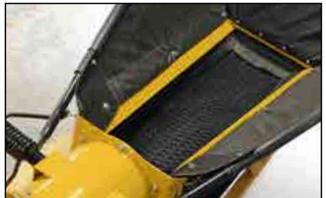
Fig 101 - Completed hopper with belt
