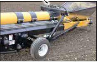
Fig 19 - Steering wheels. Check valve on cylinder mount
