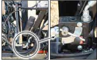
Fig 43 - Hydraulic oil flow regulator
