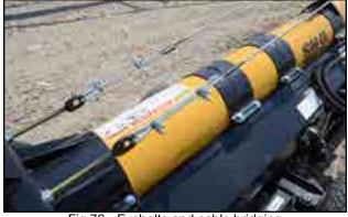
Fig 76 - Eyebolts and cable bridging
