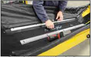
Fig 105 - Stainless steel Hold-Down Strip Plates
