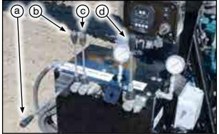
Fig 13 - Hydraulic levers
