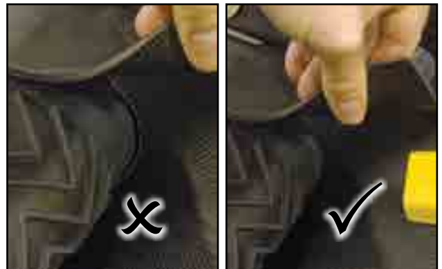
Fig 106 - Corner flashing must fit tight around the belt
