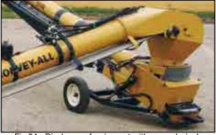
Fig 34 - Discharge of swing-out with manual winch
