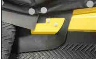
Fig 107 - Fasten flashing clamp
