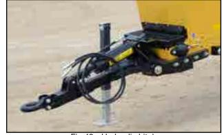
Fig 49 - Hydraulic hitch
