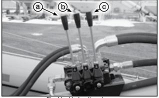
Fig 41 - Hydraulic valves
