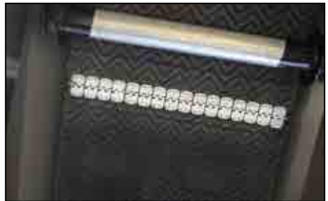
Fig 21 - Chevron belt with Alligator® lacing
