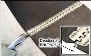
Fig 95 - Crimp lacing and taper belt corners
