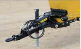
Fig 26 - 2200 series hydraulic hitch
