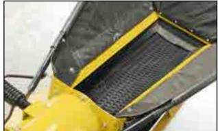
Fig 101 - Completed hopper with belt
