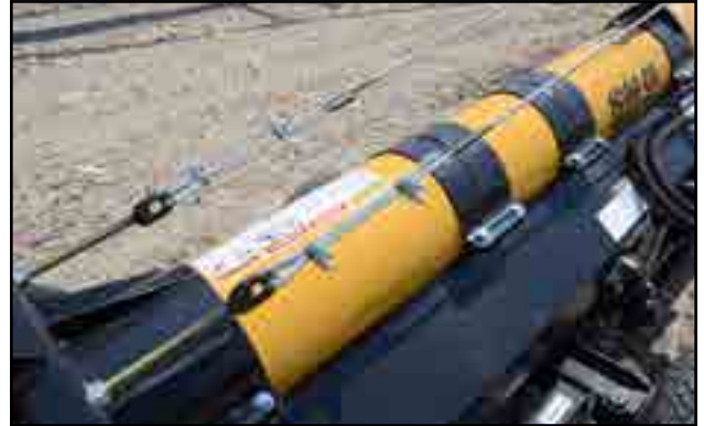
Fig 76 - Eyebolts and cable bridging
