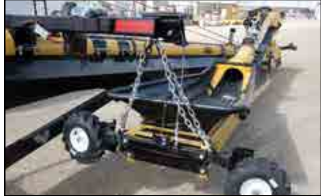
Fig 38 - Swing-out with electric mover kit
