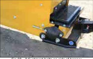
Fig 68 - Adjustment bolts on side of hopper
