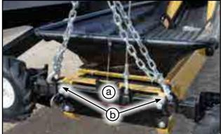
Fig 36 - 1600 series: Winch hook (a), transport hook (b)
