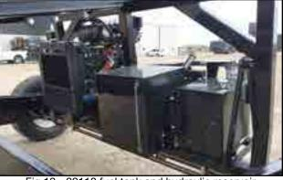
Fig 12 - 22110 fuel tank and hydraulic reservoir
