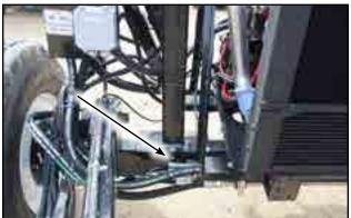
Fig 18 - Cushion block on axle, below engine
