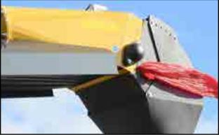
Fig 70 - discharge roller bearing
