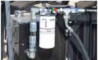
Fig 96 - Hydraulic oil filter
