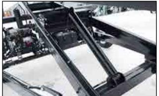
Fig 75 - Conveyor tube lift cylinder
