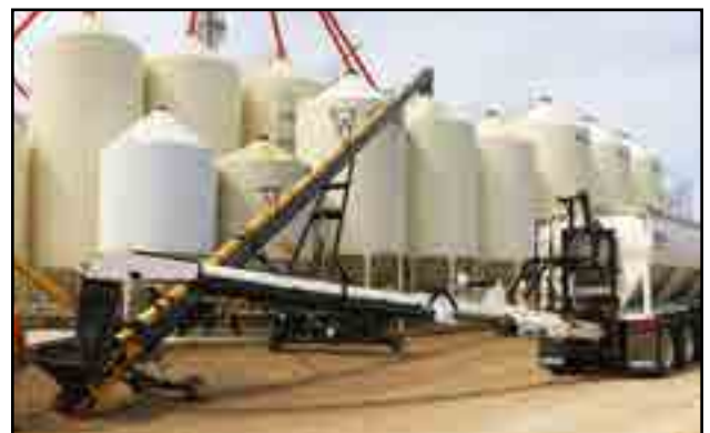
Fig 57 - CST unloading into conveyor
