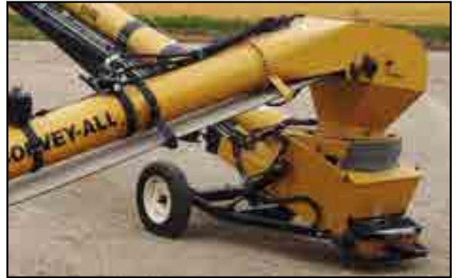
Fig 34 - Discharge of swing-out with manual winch
