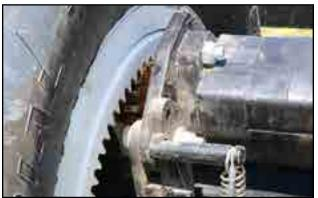
Fig 111 - Bin fill conveyor drive gears
