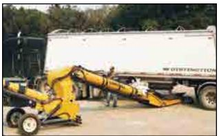
Fig 55 - Trailer unloading into swing-out conveyor
