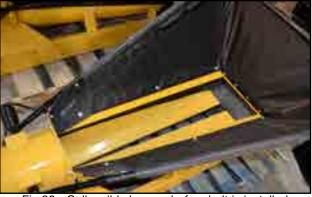
Fig 98 - Collapsible hopper before belt is installed
