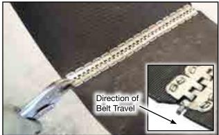
Fig 90 - Crimp lacing and taper belt corners
