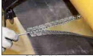
Fig 94 - Thread lacing cable
