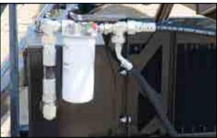
Fig 72 - Hydraulic oil filter
