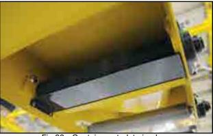
Fig 92 - Containment plate in place
