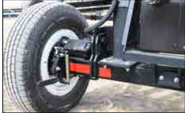
Fig 109 - Bin fill conveyor drive wheel
