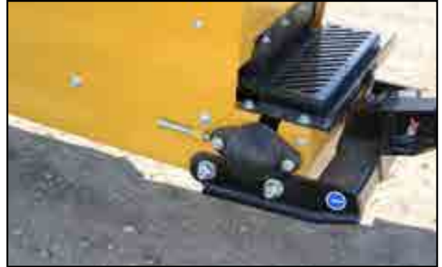
Fig 68 - Adjustment bolts on side of hopper
