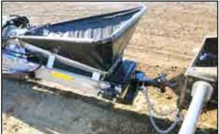
Fig 48 - Safety chain secured
