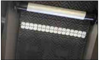
Fig 22 - Chevron belt with Alligator® lacing
