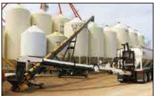
Fig 57 - CST unloading into conveyor
