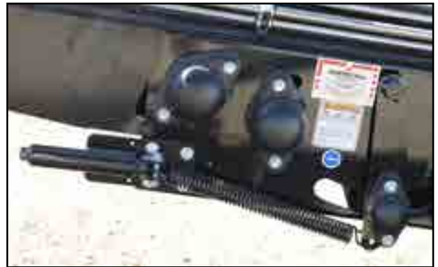
Fig 69 - Positive pinch drive tension bolts
