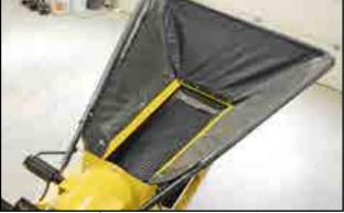
Fig 66 - Collapsible main conveyor hopper
