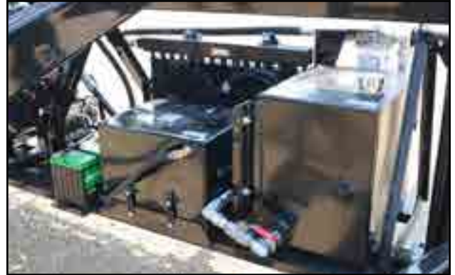
Fig 62 - Hydraulic oil reservoir and fuel tank
