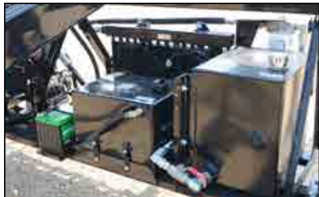
Fig 11 - 1600 Fuel tank and hydraulic reservoir
