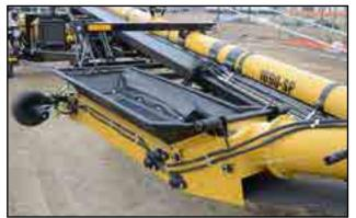
Fig 71 - Swing-out conveyor
