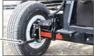
Fig 17 - Drive wheel and engagement lever
