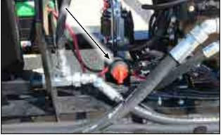
Fig 9 - Power shut-off switch
