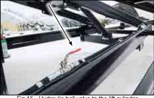
Fig 15 - Hydraulic ball valve to the lift cylinder
