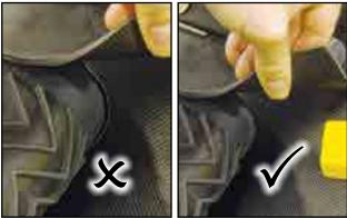
Fig 106 - Corner flashing must fit tight around the belt
