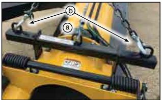
Fig 37 - 2200 series: Winch hook (a), transport hook (b)
