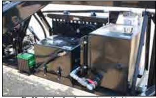
Fig 62 - Hydraulic oil reservoir and fuel tank
