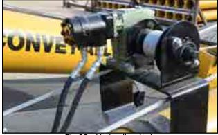
Fig 35 - Hydraulic winch
