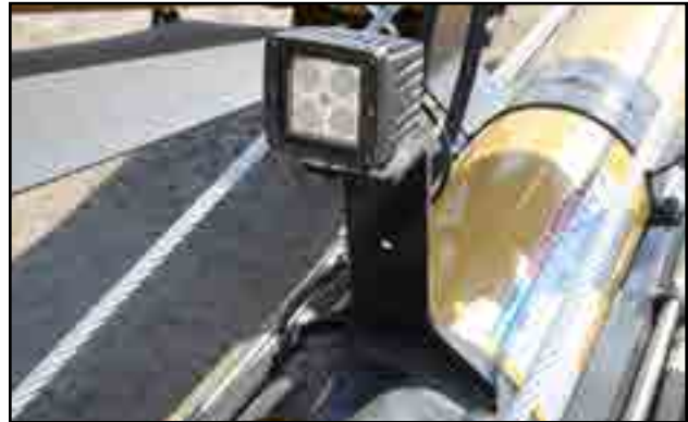
Fig 24 - Hopper working light
