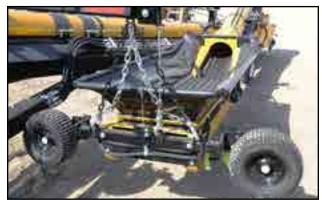
Fig 33 - Swing-out hopper wheels
