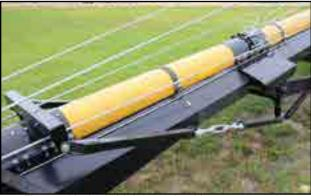
Fig 78 - Under-bridging turnbuckle on some units
