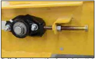
Fig 82 - Swing-out hopper idler roller and adjustment bolt
