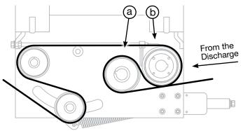
Fig 84 - Drive box, pinch roller (a) & drive roller (b)
