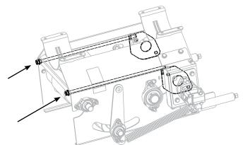
Fig 85 - Adjustment bolts and brackets inside 1600 drive box. 2200 series drive boxes do not have adjustment bolts.
