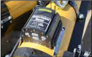
Fig 39 - Auger Jogger receiver box
