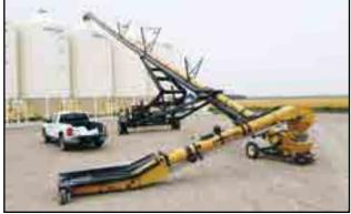
Fig 31 - Swing-out conveyor (optional)
